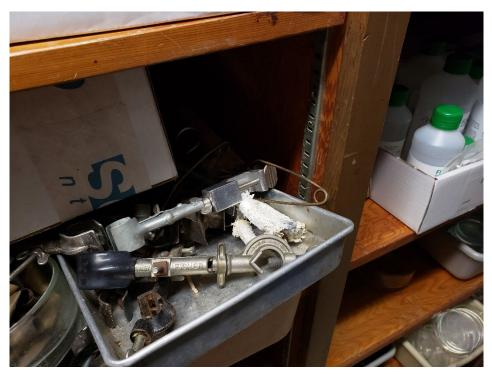
Photo 2. Asbestos Heat Pads on Beaker Holders in Science Storage Room
